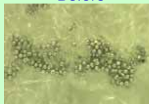
Solder particle (Diameter about 25 μm)
